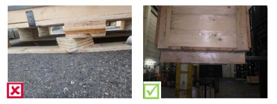
Side walls must support the load without deformation !
