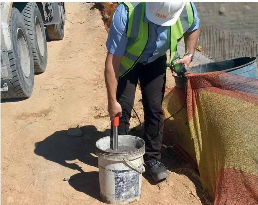
The PERI SONO w/c analyzer consists of a measuring probe and a hand-held transmitter with a display. The fresh concrete measurements are carried out in a common plastic bucket.
