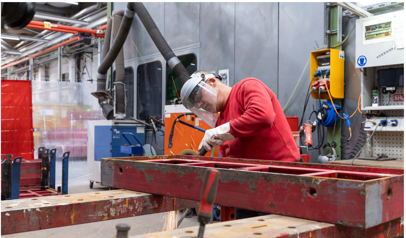
Refurbishment of a PERI formwork element.
